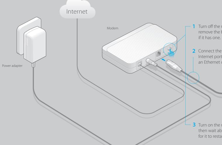
1 Turn off the modem and remove the backup battery
